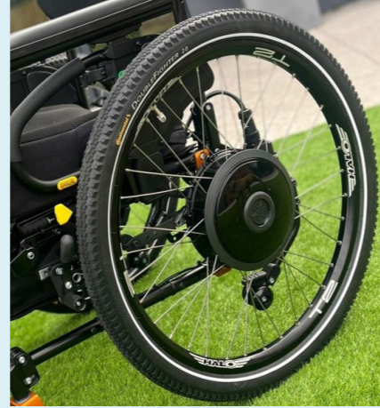
SPECIAL WHEEL BUILD WITH 24" SCHWALBE MOUNTAIN BIKE TYRES AND TANNUS INSERTS
