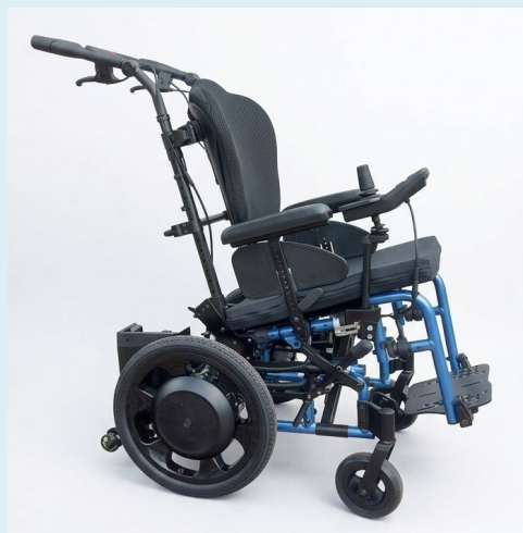
16" SD MOTION DRIVE SYSTEM (FITTED TO A LITTLE WAVE ARC WHEELCHAIR)
